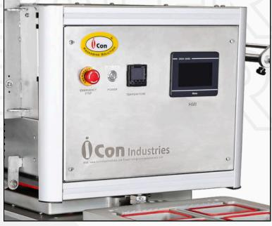
A Rotary Tray Sealer is a semi-automated packaging system that uses a rotating table to seal trays with a film cover. It allows for efficient sealing with the ability to handle multiple tray sizes, ideal for small to medium production runs. It removes air from the package to extend shelf life by reducing exposure to oxygen, preserving freshness and preventing spoilage.
